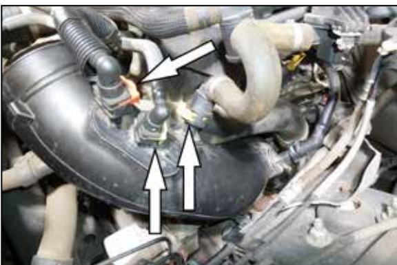
9. Release the locks that secure the vent lines to the ejector fitting and CCV fitting, then disconnect the lines from the fittings.
