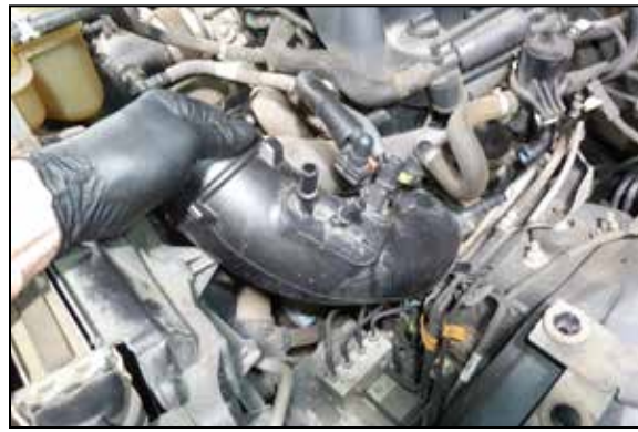
11. Loosen the hose clamp at the turbo inlet, unhook the mounting post and remove the driver side turbo inlet tube and then remove the driver side inlet tube from the vehicle.
