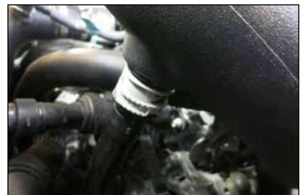
17. Connect the BOV hose to the BOV fitting installed into the K&N tube. Be sure the hose is locked into position with the locking ring.
