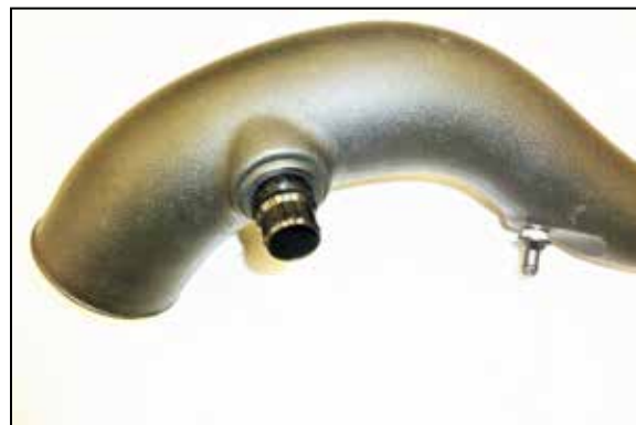
13. Install the grommet and BOV fitting into the driver side K&N turbo inlet tube. Apply a small amount of lubricant onto the fitting to ease installation.
