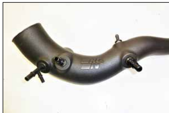
14. Install the provided CCV fitting and mounting stud into the K&N driver side turbo inlet tube. Install the provided ejector fitting into the K&N driver side turbo inlet tube using the provided grommet.
