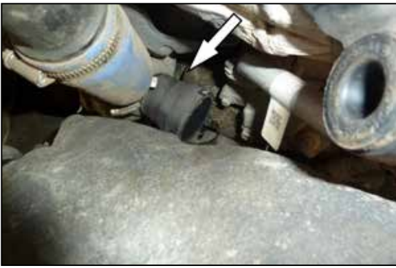
6. Install one of the provided step couplers onto the turbo inlet and secure with the provided hose clamp.
