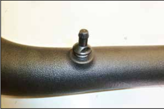
7. Install one of the provided mounting studs onto the K&N tube using the provided stud and aluminum spacer as shown.
