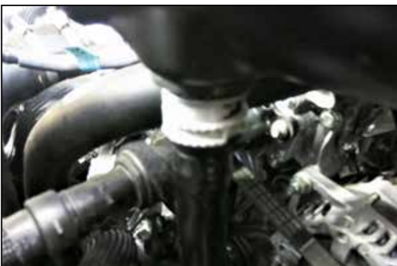
10. Rotate the BOV locking ring counterclockwise and then disconnect the BOV hose from the turbo inlet tube.
