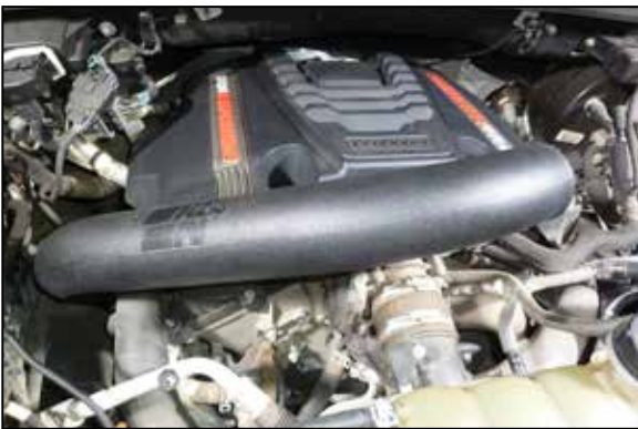
8. Place the K&N passenger side turbo inlet tube into position in the coupler and so the mounting stud aligns with the mounting grommet. Secure the tube with the hardware and clamp provided.
