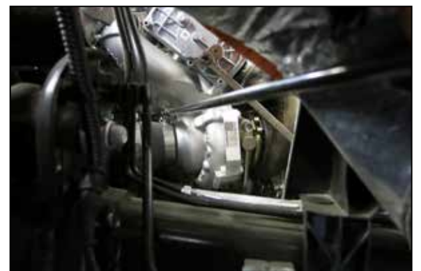
16. Install the K&N driver side turbo inlet tube so the coupler attaches to the turbo inlet and the mounting stud engages the mounting grommet. Secure the tube with the provided hardware and hose clamp.
