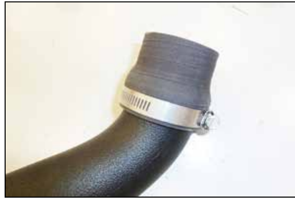
12. Install the provided step coupler and hose clamps onto the K&N driver side turbo inlet tube.
