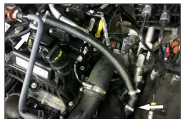
19. Remove the factory CCV hose assembly from the valve cover and install the CCV hose assembly onto the valve cover and turbo inlet tube fittings.
