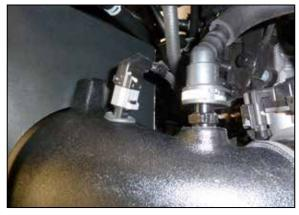
13. Reconnect the IAT sensor electrical connection and connect the CCV line to the fitting.
