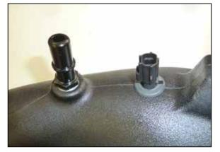
11. Remove the IAT sensor from the factory intake tube, remove the O-ring from the sensor and then install it into the K&N intake using the provided grommet. Apply thread sealer to the CCV fitting and then install the fitting into the K&N intake tube.
