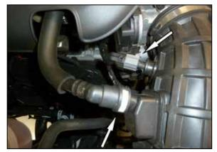
2. Disconnect the IAT sensor electrical connection. Disconnect the CCV fitting from the intake tube.
