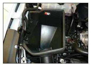
9. Install the K&N heat shield into the vehicle so the mounting pins insert into the mounting grommets and the fresh air intake fits inside the opening.
