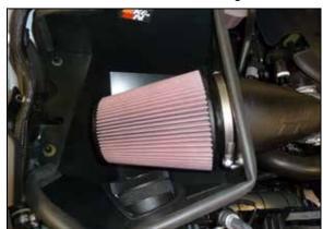
14. Install the Air filter onto the intake tube and secure with the provided hose clamp.
