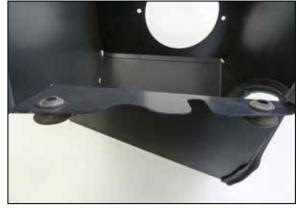
8. Remove two mounting grommets from the stock air filter housing and install them into the K&N heat shield as shown.
