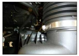
4. Loosen the hose clamp that secures the intake tube to the air filter housing and then remove the intake hose from the vehicle. 5. Pull the air filter housing up to disengage it from the mounting grommets and then remove it from the vehicle.
