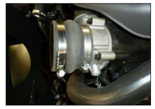
10. Install the provided hump coupler onto the throttle body and secure with the provided hose clamp.
