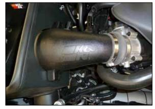
12. Install the K&N intake tube into the coupler and then into the heat shield, align the tube in the heat shield and secure with the provided hardware and hose clamp.
