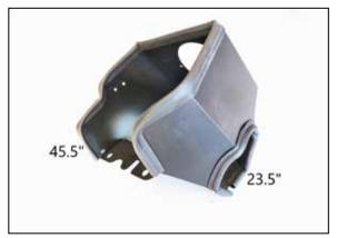
6. Cut the edge trim into one section of 45.5' length and one of 23.5" long. Install the edge trim onto the heat shield as shown.
