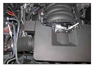
3. Loosen the hose clamps that secure the intake plenum to the throttle body and air filter housing. Then remove the intake plenum from the vehicle.
