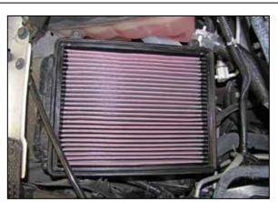
5. Install the K&N® air filter into the lower filter housing and then reinstall the upper housing and secure with the factory hardware.
