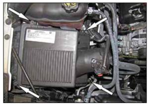
4. Loosen the screws that secure the upper air filter housing and then lift off the housing to remove the factory air filter.
