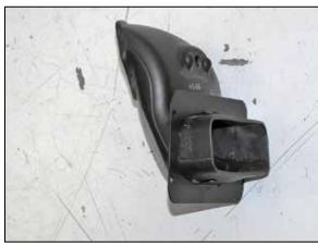
23. Install the provided bracket (064339) onto the fresh air duct as shown.
