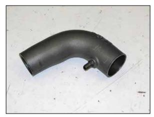
30. Install the provided NPT crank case vent fitting into the  $K\&N^{\mbox{\tiny 0}}$  intake tube as shown.
