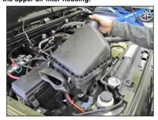
5. Lift up the air filter housing to dislodge it from the mounting grommets and then remove it from the vehicle.
