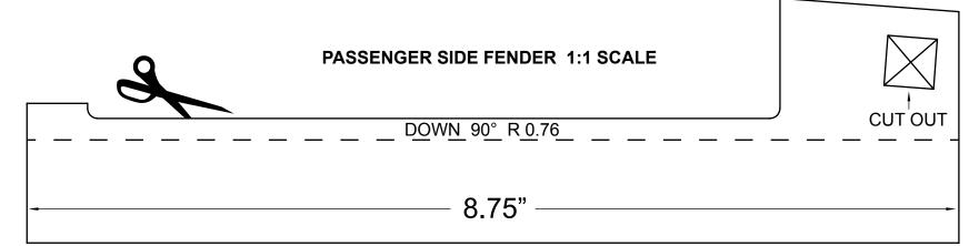
Carefully cut along outer edge of template and also cut out the square alignment hole.
