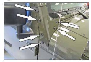
7. Using a T40 socket, remove the six bolts that secure the corner cap and then remove the corner cap
