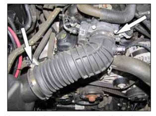
3.Loosen the hose clamps securing the intake tube.
