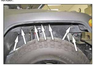
15. Remove the seven inner fender bolts.
