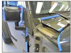
18. Reinstall the corner cap and secure with the factory hardware.
