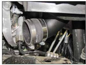
39. Install the provided coupler (08284) onto the elbow secured to the air filter housing and secure with the provided hose clamp.
