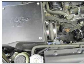
28. Install the provided hump coupler (08699) onto the filter adapter and secure with the provided hose clamp.
