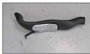
38. Install the provided heat shield and mounting bracket (064339) onto the K&N<sup>®</sup> lower tube as shown using the provided hardware.
