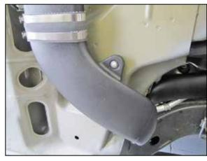
52. Secure the corner tube with the provided sheet metal screw into the hole previously drilled.
