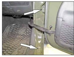
12. Loosen the two fender bolts inside the passenger door jamb.
