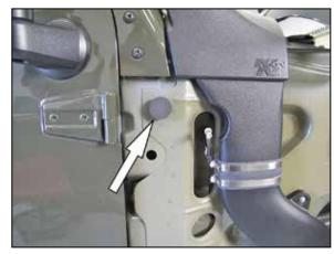
54. Peal the backing of the provided damper pad and then install it as shown on the inner body.
