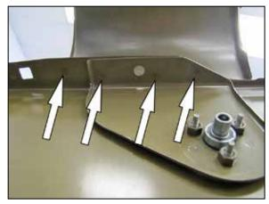
45. Use a center punch to mark the four spot welds which hold the cowl corner cap to the fender. Then drill out the spot welds to remove the cowl cap from the fender.
