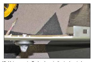
48. Using a cut-off wheel or similar tool, cut along the lines marked with the template and remove that section of the fender. Be sure to remove any remaining burrs with a file or deburring tool.
