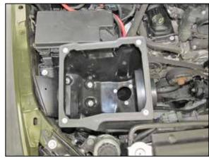
25. Install the air filter housing assembly into the vehicle onto the insert nuts and secure with the provided hardware.
