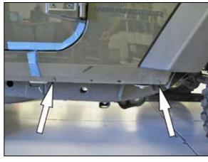
13. Remove the two lower fender bolts.
