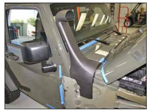
42. Temporarily install the snorkel and secure with the factory cowl bolts.
