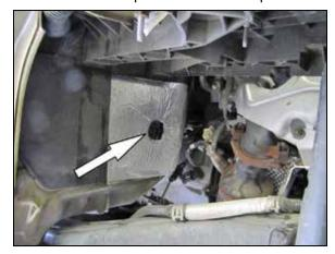
36. Remove the Insulation retaining nut shown.
