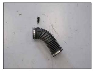
32. Remove the inlet air temperature sensor from the factory intake tube.
