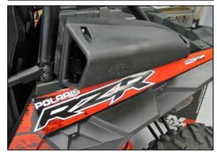
6. Install the K&N® prefilter/scoop assemblies onto the vehicle and secure with the provided hardware.
