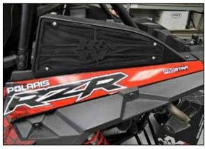
8. OPTION #2 Additional shorter hardware has been included so the pre-filters can be run without the scoops if desired. Be sure to use the cage supports for the pre-filter if the scoops are not used.
