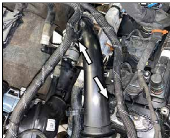
2. Disconnect the coolant hoses from the hot-side charge tube.
