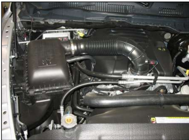
Factory air box system installed
