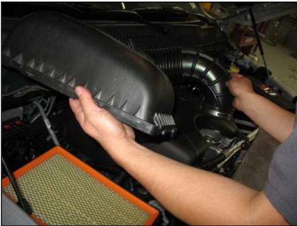
g. Unclip the air box lid from the air box base.
