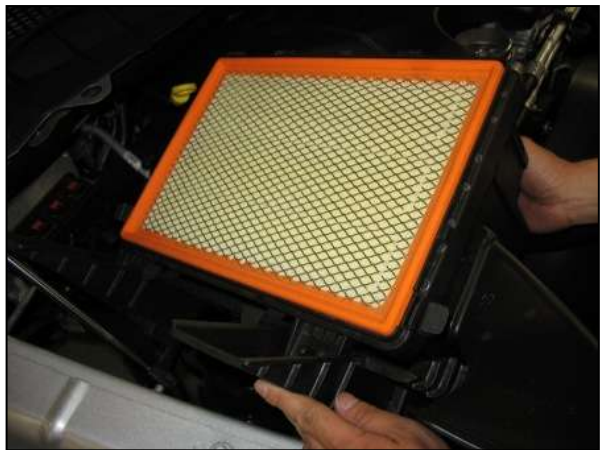
j. Remove the air box base and air filter from the vehicle.
