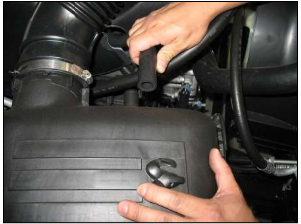
f. Disconnect engine breather hose at the air box lid.
