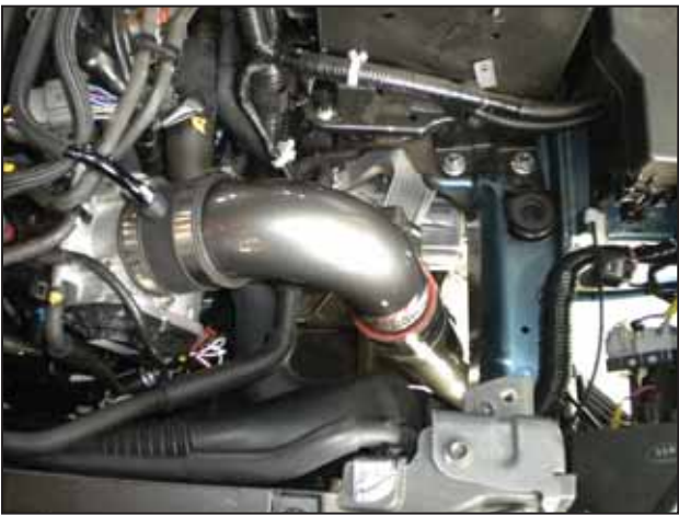
j. Upper intake pipe bracket secured to the coolant hose.
