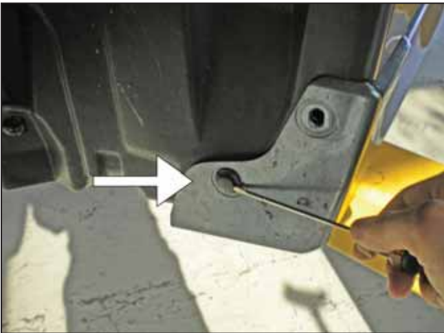
e. Remove the plastic wheel liner. This liner is held in by 16 plastic clips as shown. To remove plastic clips use a Phillips end screw driver to remove the plastic screw in the center, then pull out the clip. A pick or flat blade screw driver can be used for popping out the two clips used in the bottom corner toward the rear of the wheel well.
