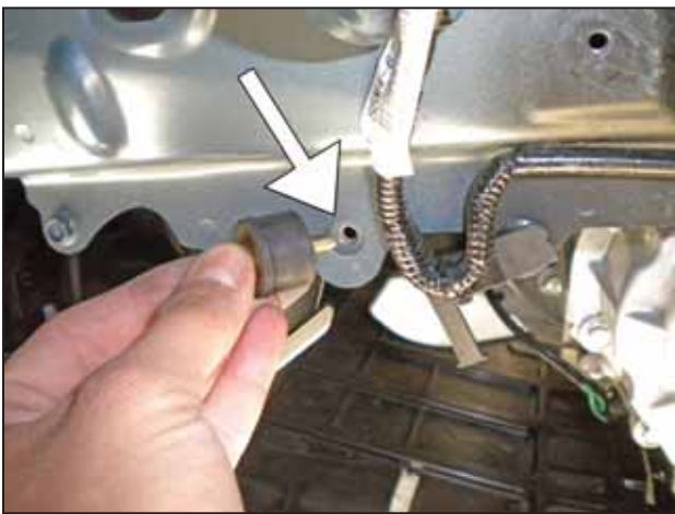
f. Install the threaded soft mount into the location shown.
