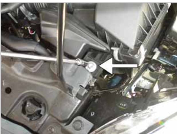
k. Remove the 10mm bolt attaching the air cleaner box to the core support.
