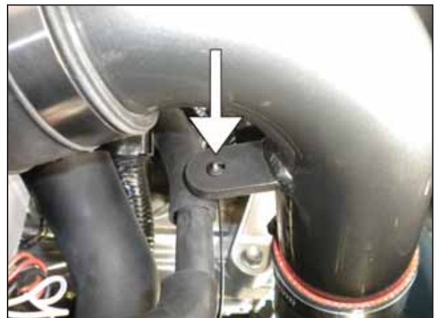
i. Secure the coolant hose to the bracket on the upper intake pipe with the supplied tree mount zip tie.
