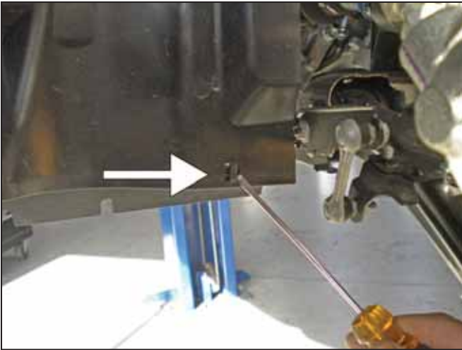
c. Undo the plastic clip at the bottom.
