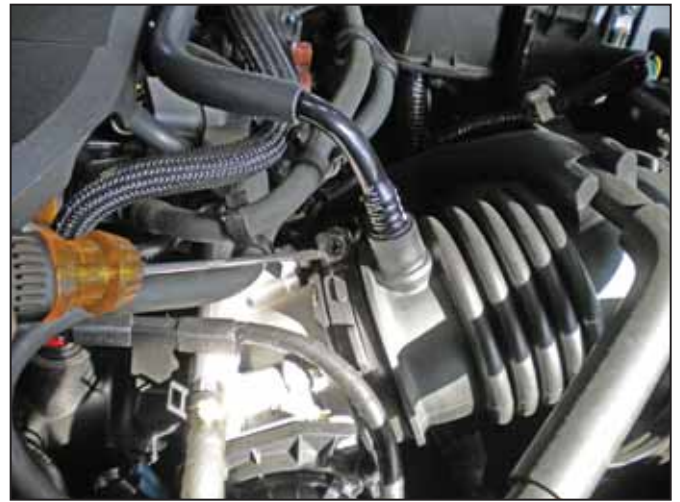
h. Loosen 10mm hose clamp fastener just enough in order to remove the rubber boot over the throttle body.
