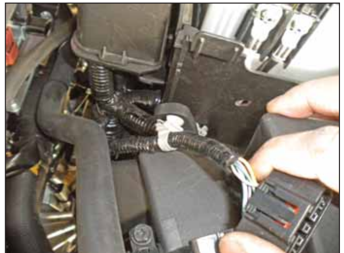
j. Undo the grey plastic clip to the harness.
