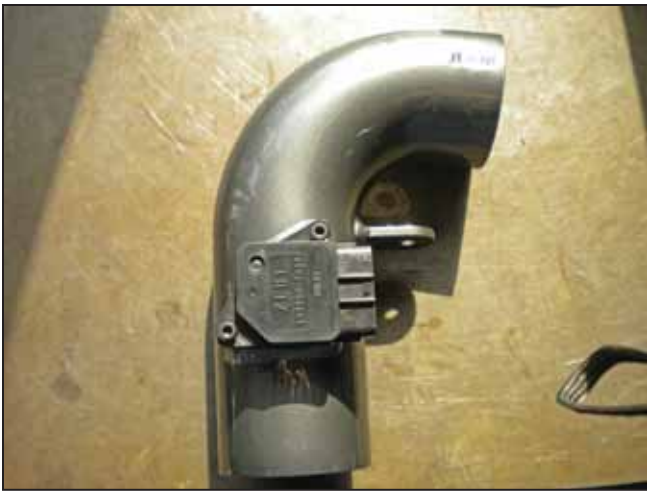
d. Install the MAF sensor into the upper intake pipe using the supplied bolts.
