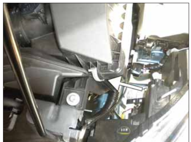
l. Undo the 2 metal retaining clips holding the air box lid.
