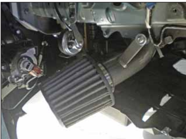
h. Attach the AEM® air filter onto the lower intake pipe with a size 44 hose clamp.
