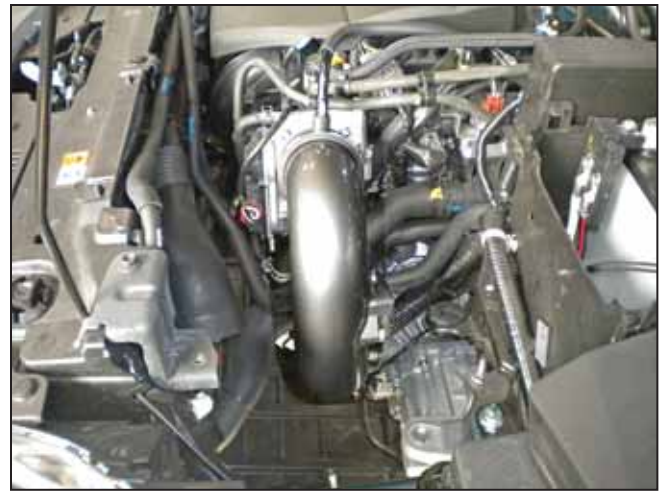
e. Install the upper intake pipe onto the coupler installed earlier in step 3b.
