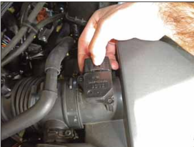
i. Remove the Mass Air Flow sensor harness by pressing down on the tab and pulling it off.
