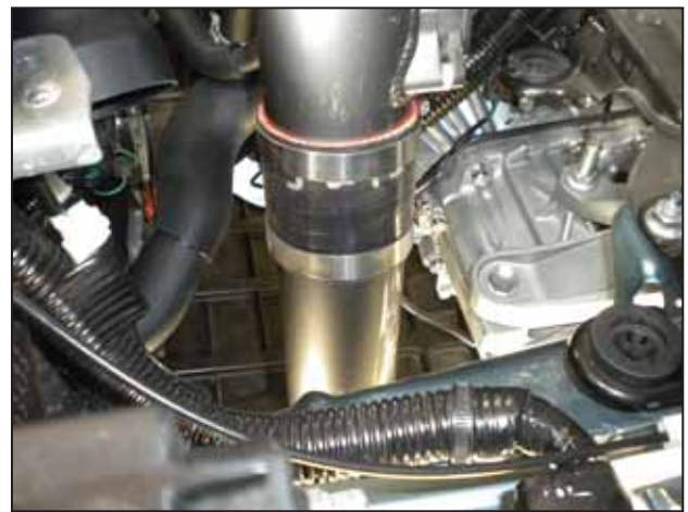
g. Use the 2.75"x3" coupler to attach the lower pipe to the upper pipe, using the supplied size 44 hose clamps. Fasten the bracket to the threaded soft mount with the supplied nut and bolt.
