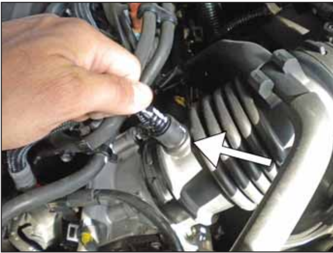
g. Pull out the PCV hard line from the nipple located just in front of the throttle body.
