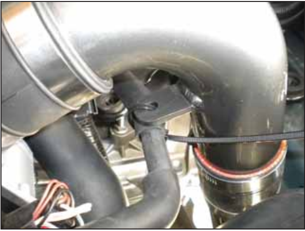
j. Upper intake pipe bracket secured to the coolant hose.
