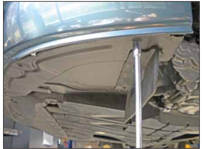
f. Remove the three 8mm bolts/screws along the outer edge of the front portion of the wheel liner on the driver side.
