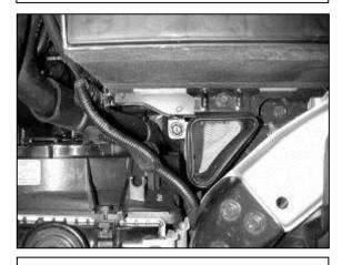
h. Remove the bolt securing the lower resonator box.
