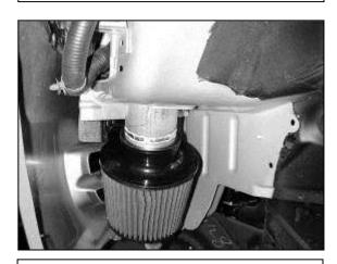
j. Install the air filter and secure using the 9452 hose clamp.
