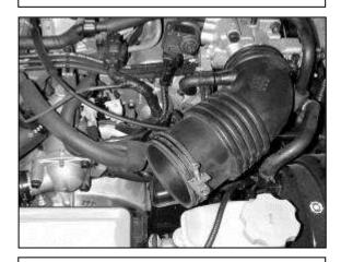
f. Remove the air flow sensor from the stock inlet pipe and set aside. Do not unplug the sensor. Remove the hose clamps securing the stock inlet pipe in place. Remove the breather tube and stock inlet pipe from the vehicle.
