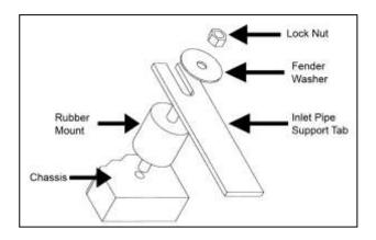
Proper installation of the rubber mount assembly
