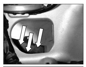
c. The area that needs to be trimmed / enlarged is the area below the actual opening as the arrows depict. Ensure that any rough or sharp edges are smoothed and that the AEM® intake pipe is able to clear the opening without touching any part of the inner fender.
