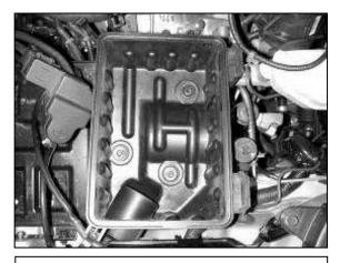
d. Remove the filter from the lower filter box. Remove the three bolts securing the lower box and remove.
