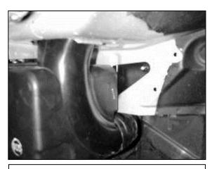
i. Remove the nut securing the lower resonator in place.
