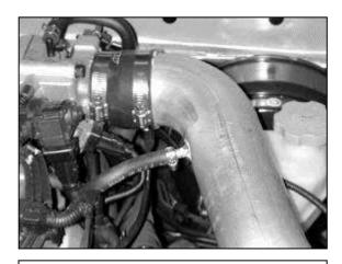
d. Install the upper inlet pipe in the vehicle. Use the reducer coupler, 9448, and 9444 hose clamp to secure the inlet pipe in place. Install the new breather hose and secure with the 4093-5 hose clamps.
