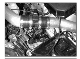
h. Install the second 3" coupler onto the lower intake pipe and secure in place with a 9448 hose clamp. Insert the coupler of the lower intake pipe onto the air flow sensor and secure with the remaining 9448 hose clamp. Ensure the lower intake pipe's bracket aligns with the rubber mount previously installed. Install the washer and nyloc nut to secure the inlet pipe bracket to the rubber mount.
