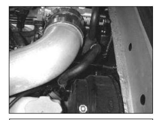
e. Remove the brake booster vacuum line hose clamp and push the vacuum hose down completely over the metal nipple. Reinstall the hose clamp and ensure there is adequate clearance for the intake pipe.
