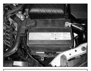
b. Disconnect the negative and positive battery terminals. Remove the battery from the engine compartment.
