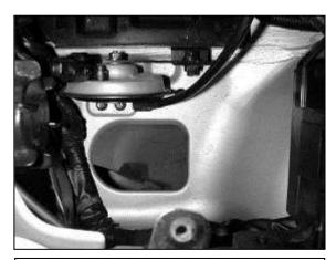
b. The factory hole that the inlet pipe passes through must be enlarged for clearance of the AEM® intake pipe. The use of a specialized power tool will be needed to cut through the inner fender so the AEM® intake pipe is able to clear the inner fender opening.
