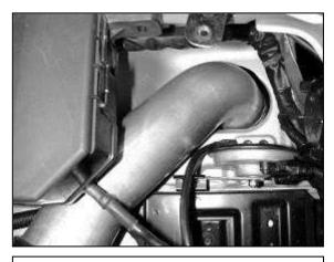
i. The lower intake pipe will pass through the hole in the fender well. Ensure that the intake pipe does not contact any part of the body.
