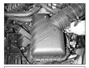
c. Remove the hose clamp securing the filter box top to the air flow sensor. Unclip the filter top box and remove.
