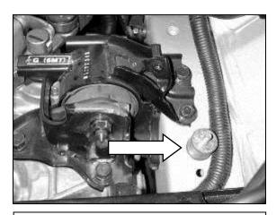
g. Install the soft rubber mount in the threaded hole exposed from the removal of the mounting bracket in step 2e.
