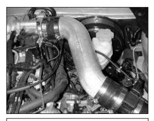
f. Install one of the 3" couplers on the end of the upper inlet pipe and secure with a 9448 hose clamp. Install the air flow sensor into the coupler and secure with a 9448 hose clamp.
