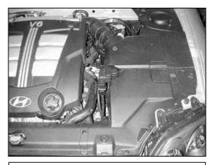
a. Remove the plastic covers covering the stock air box system and battery.
