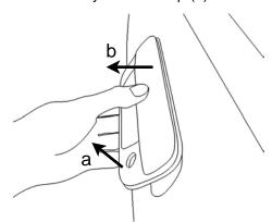
5 Install the Pop & Lock assembly into the tailgate following Steps 2, 3 & 4 in reverse order while making sure that it is in the lock position as seen in picture below. Make sure that the bottom small tabs snap onto the tailgate before tightening the 6 mm bolts.
