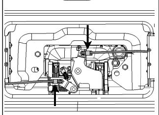
**3** Remove the two 6 mm bolts from inside of the tailgate to free the handle assembly.
