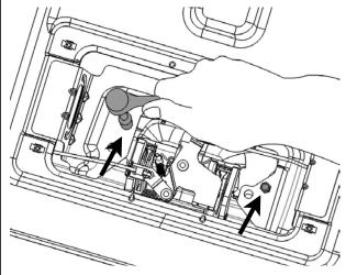
4 Lift the tailgate into the up position but do not fully engage in the latches. While supporting the tailgate with one hand, pull the bottom of the handle out first (a), then carefully pull out the handle assembly from the top (b).
