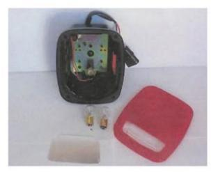
Step # 2 Insert new reflector, line up tabs on both sides of housing, reflector may be snug, but will slide in tightly.
