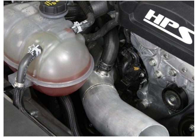
11. Re-attach the bypass valve re-circulator hose onto the HPS intake pipe.
