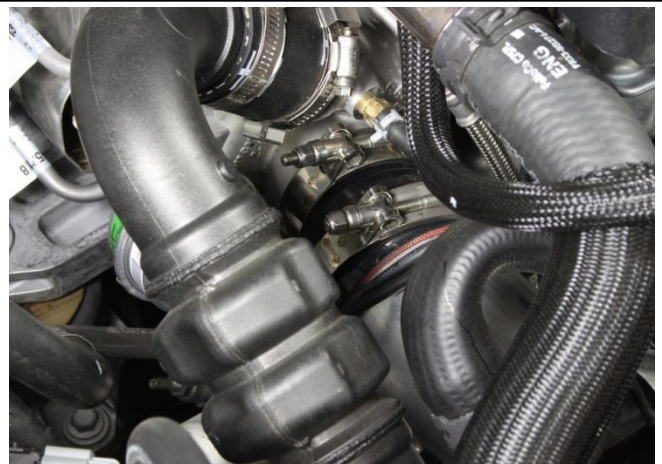
9. Install the silicone reducing coupler onto the turbo inlet along with the T-Bolt clamps included. Then install the HPS intake pipe onto the silicone coupler.
