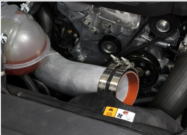
12. Install the straight silicone coupler onto the end of the first HPS intake pipe.
