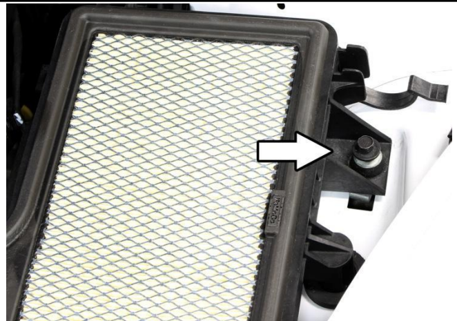
7. Remove the bolt attaching the lower portion of the air box to the body using a 10mm socket.
