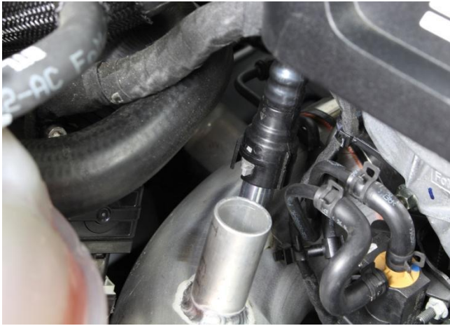
10. Clip in the PCV connector onto the port on the HPS intake pipe.
