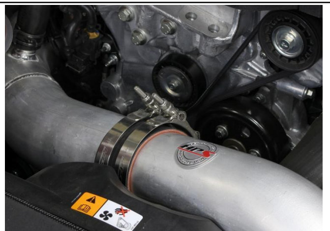
17. Attach the HPS intake pipe to the silicone coupler, connecting the two pipes together.
