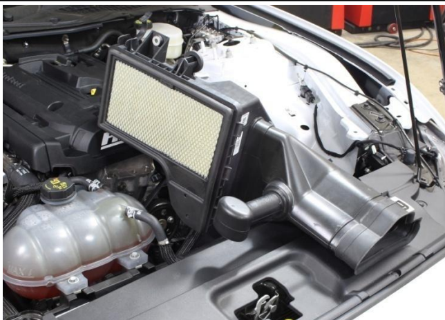
8. Remove the lower portion of the air box from the engine bay.
