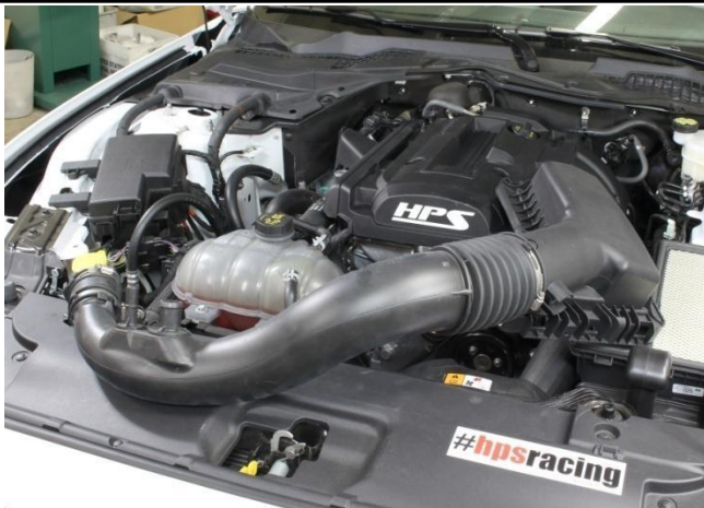
6. Remove the air box and intake elbow from the engine bay.
