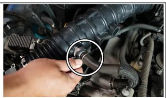
3. Loosen the clamp securing the breather hose from the factory intake tube and disconnect the hose from the intake barb.
