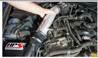
9. Insert the HPS intake pipe into the throttle body side coupler, then into the airbox coupler. Secure the retaining buckles back onto the air box assembly, then adjust the intake pipe into the proper position and secure all the hose clamps.
