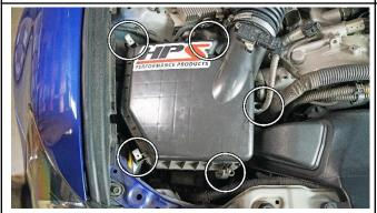
4. Release the four retaining buckles securing the top portion of the air box.
