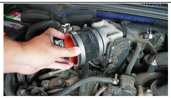
7. Install and secure the silicone coupler onto the throttle body using the supplied EMSC clamps.
