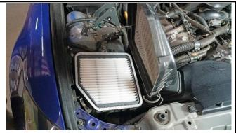
6. Remove the factory air filter and insert the HPS performance panel air filter into the air box assembly.
