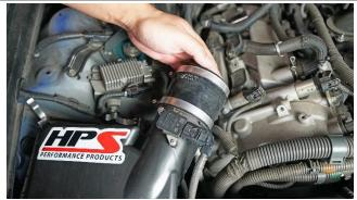
8. Install and secure the silicone coupler onto the air box using the supplied EMSC clamps.
