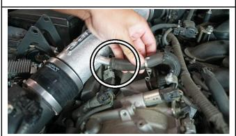
10. Re-secure the breather hose onto the intake barb.
