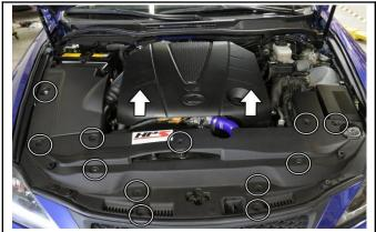
2. Lift and remove the engine cover from the vehicle. Remove the 12 plastic clips securing the air box cover and the radiator cooling panel. Remove the panels from the vehicle.
