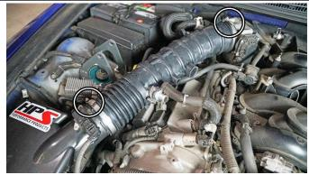
5. Loosen the hose clamps securing the intake hose from the throttle body and the air box. Remove the factory intake hose from the vehicle.
