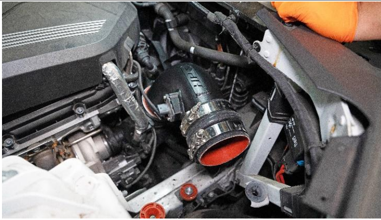
15. Insert the HPS intake into the reducer coupler.
