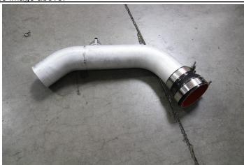
8. Install and secure the provided reducer coupler onto the end farthest away from the MAF flange using the T-bolt clamp SSTC-79-87.
