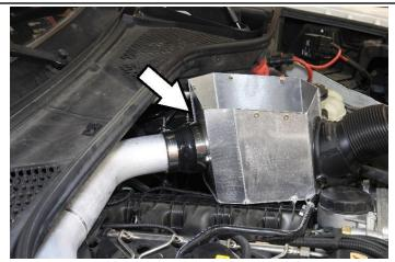
12. Insert the HPS heat shield into the vehicle and into the reducer coupler. Connect the rubber grommet onto the factory air box mount. Reconnect the factory air duct into the heat shield.
