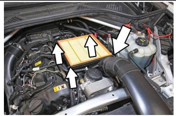
5. Lift the lower air box assembly from its grommets, then disconnect the lower air box from the air duct. Remove the lower air box assembly from the vehicle.
