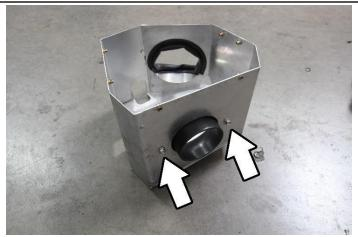
6. Install and secure the provided velocity stack into the heat shield using the two M6x12mm bolts and washers.
