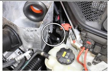
13. Install and secure the provided bracket onto the heat shield using the M6x16mm bolt, nut, and washers.
