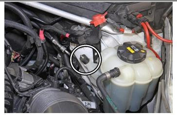
10. Remove the existing 10mm bolt securing the coolant reservoir tank and replace it with our 1-inch vibration mount.
