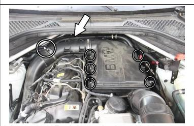
3. Loosen the 6x Torx bolts securing the upper air box assembly. Loosen the hose clamp securing the stock air intake tube. Disconnect the mass air flow sensor harness connector and carefully lift the stock air intake tube from its grommet.
