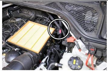
4. Disconnect the three rubber harness mounts from the lower air box assembly.
