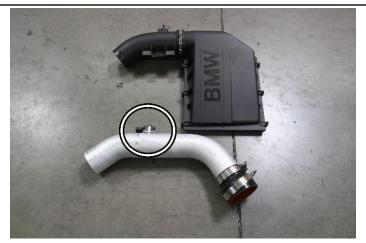
9. Remove and secure the mass air flow sensor using the provided M4x8mm allen bolts.
