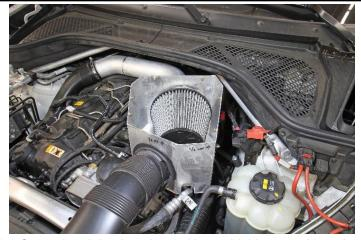
14. Once, the air intake tube and heat shield are positioned properly, tighten down the T-bolt clamp, hose clamp, and bracket. Insert the provided HPS performance air filter.
