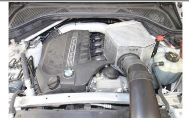
16. Insert the engine cover back into the vehicle using the factory rubber inserts from the factory intake tube.
