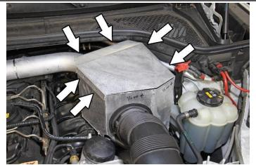
15. Insert and secure the heat shield lid onto the heat shield using the provided M5x12mm bolts.
