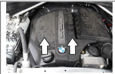
2. Lift and remove the engine cover from the vehicle.
