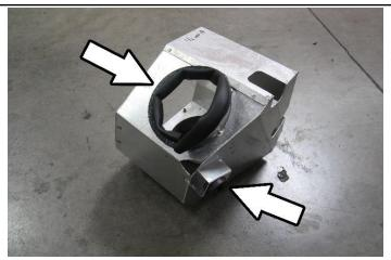
7. Remove one of the factory rubber grommets from the lower air box assembly and insert it into the HPS heat shield. Install the provided bubble edge trim onto the heat shield shown in the image above.
