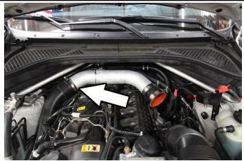
11. Reconnect the mass air flow sensor harness connector and loosely insert the HPS intake tube into the air inlet tube.
