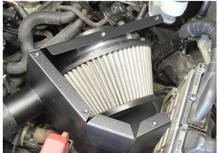
17. Carefully slide the HPS air filter in place and secure it to the velocity stack.
