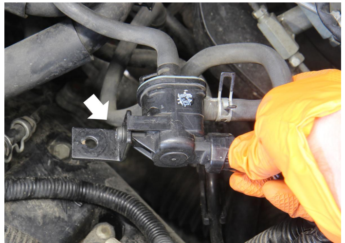
13. Install the L bracket onto the EVAP valve using the original phillips head screw.
