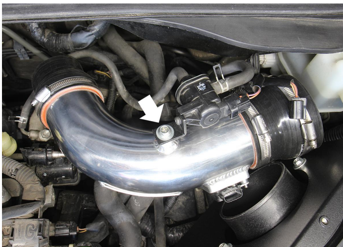
18. Place the intake pipe on its side into the engine bay and fasten the L bracket and EVAP valve onto the intake pipe.
