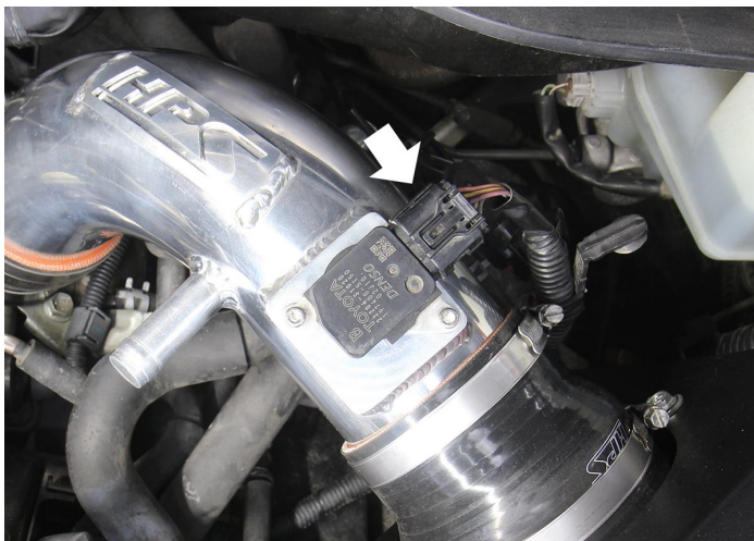
20. Reconnect the MAF sensor.
