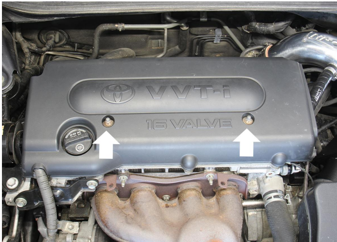
22. Reinstall the plastic engine cover.
