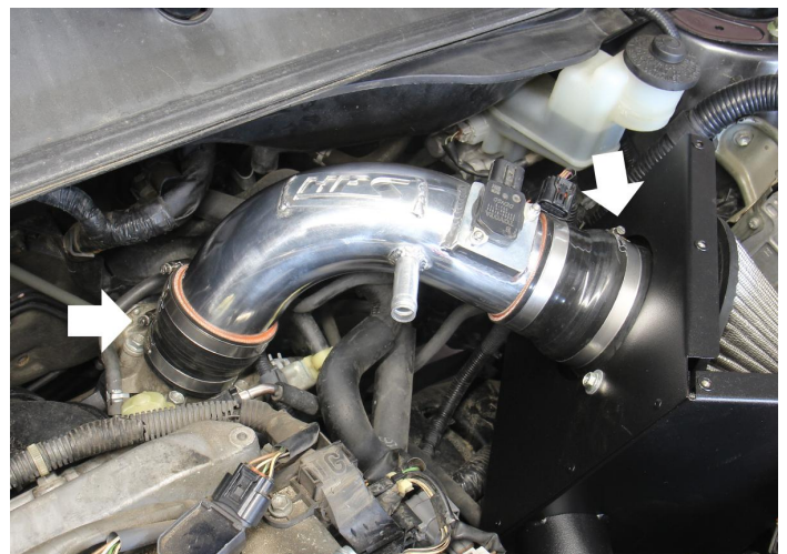
19. Slip the silicone reducers into position on the throttle body and velocity stack, then fasten the clamps to secure the pipe.
