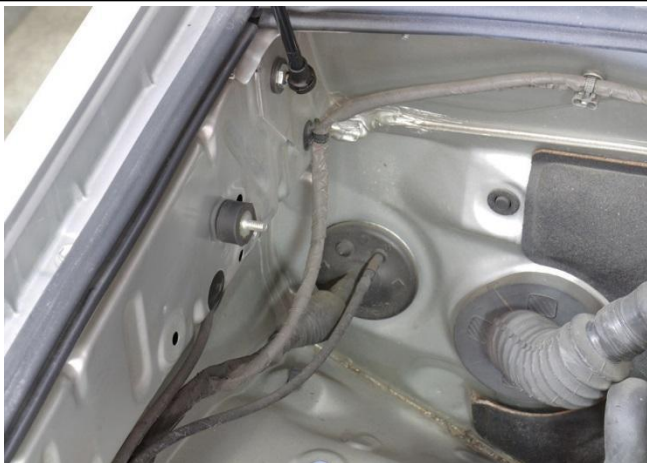
14. Install the 1/2" vibration mount into the location where the ground wire was removed.
