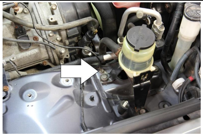
13. Mount the ground wire located in the image above reusing the factory ground bolt.
