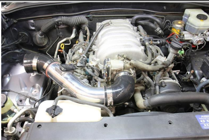
20. Install the pre-assembled intake onto the throttle body. *Do not tighten clamps yet because you will need to readjust the intake later on.
