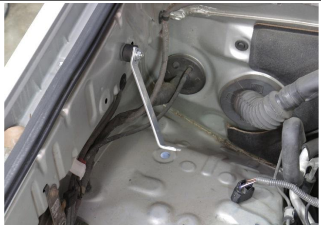
15. Install the longest heat shield bracket onto the rubber mount.
