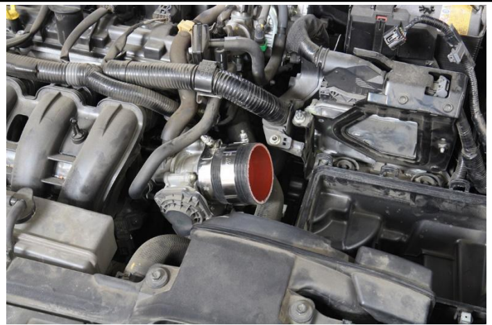
9. Install the reducer coupler along with the provided T-bolt clamps onto the throttle body.
