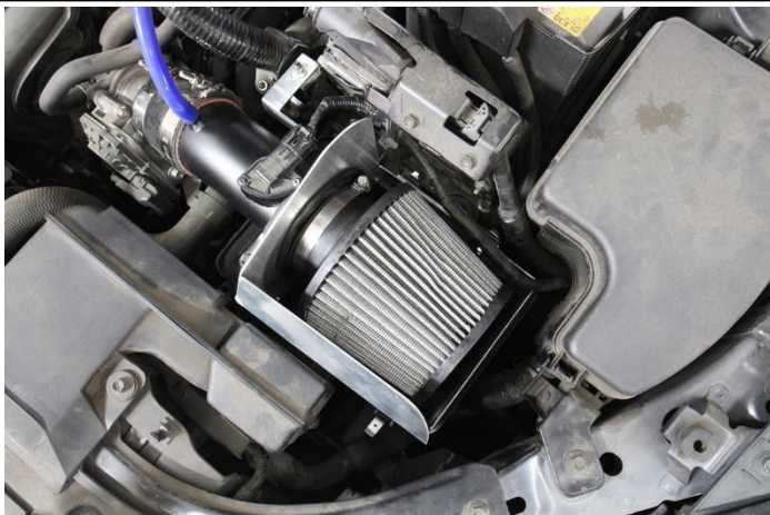
22. Install the HPS performance air filter and reinstall the engine cover back into the vehicle.
