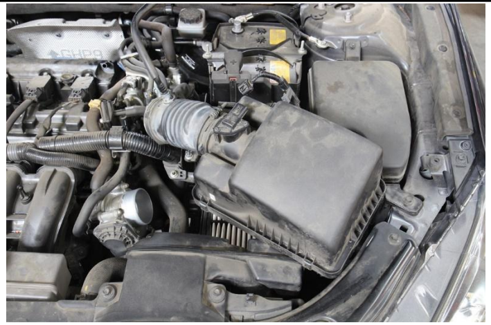
7. Remove the upper air box assembly along with the factory intake tube from the vehicle.
