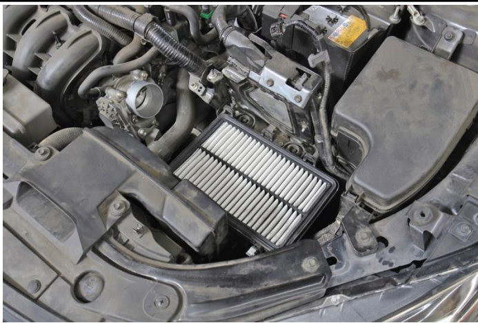
8. Remove the air filter from the vehicle.
