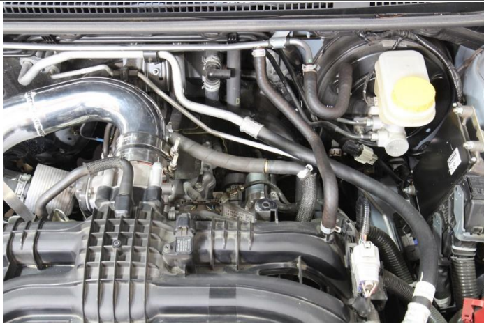
22. Insert the provided joiner into the factory breather hose. Install and secure the EPDM hose onto the provided joiner and intake barb using the EMSC-12-22 clamps.
