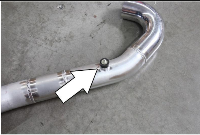
16. Install the provided vibration mount onto the HPS intake pipe.
