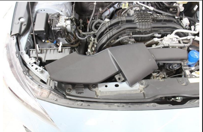
9. Disconnect the factory air duct from the lower air box and remove the air duct from the vehicle.
