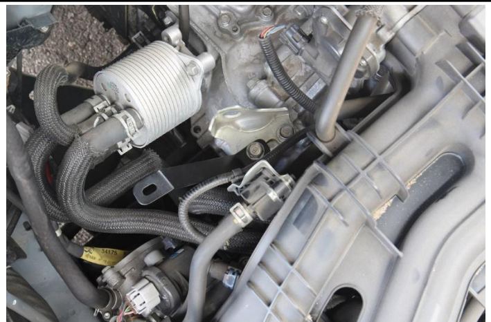
19. Insert and loosely secure the provided intake bracket by reusing the 14mm bolt.
