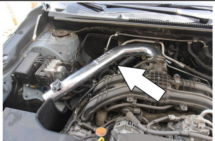
21. Insert the HPS intake pipe into the throttle body coupler and secure the vibration mount onto the intake bracket using the provided M6 nut.
