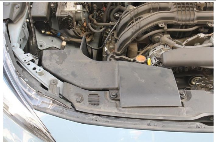
15. Install the factory air duct back into the vehicle.
