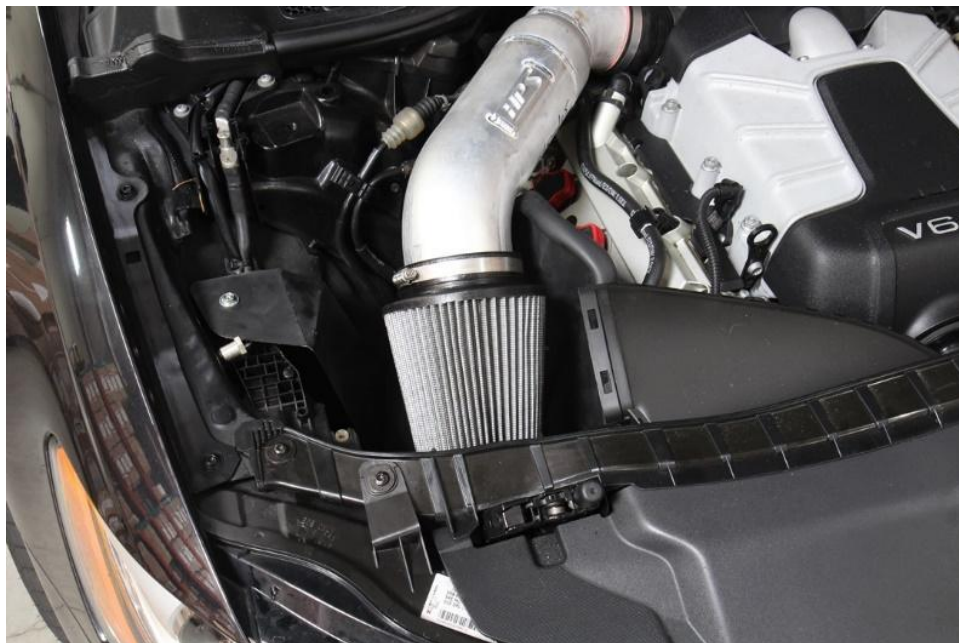
18. Install the HPS Performance Air Filter onto the intake pipe.
