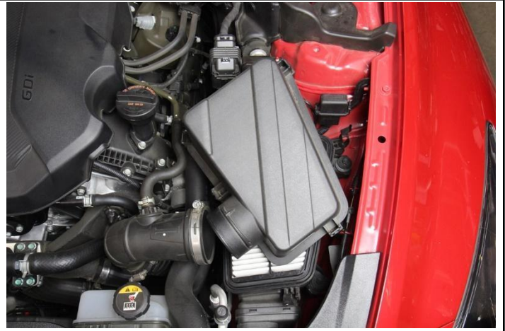
11. Separate the upper air box from the intake tube and remove the upper air box from the vehicle.
