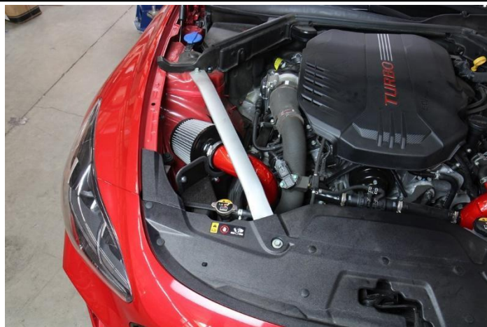
38. Reinstall the passenger side strut tower brace onto the vehicle.
