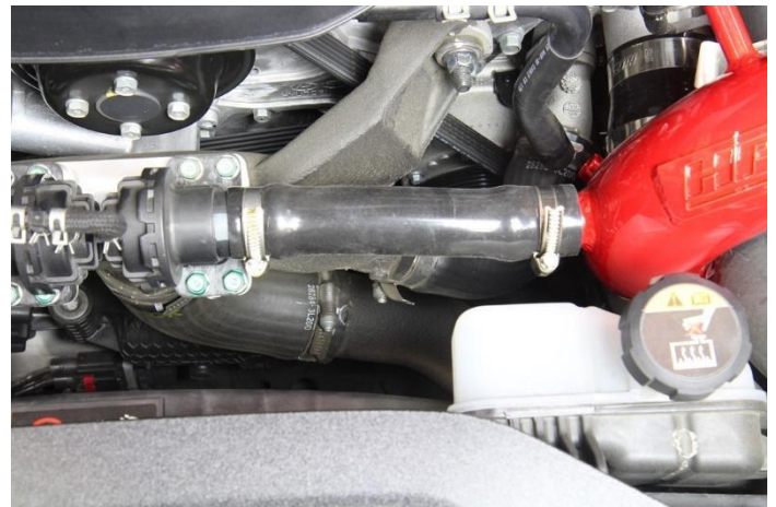
25. Insert the hose into the BOV outlet and secure the hose with the provided hose clamp.
