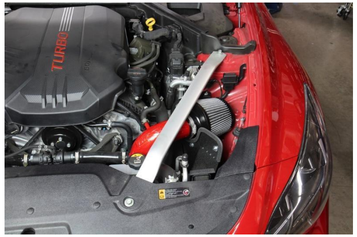
37. Reinstall the driver side strut tower brace onto the vehicle.
