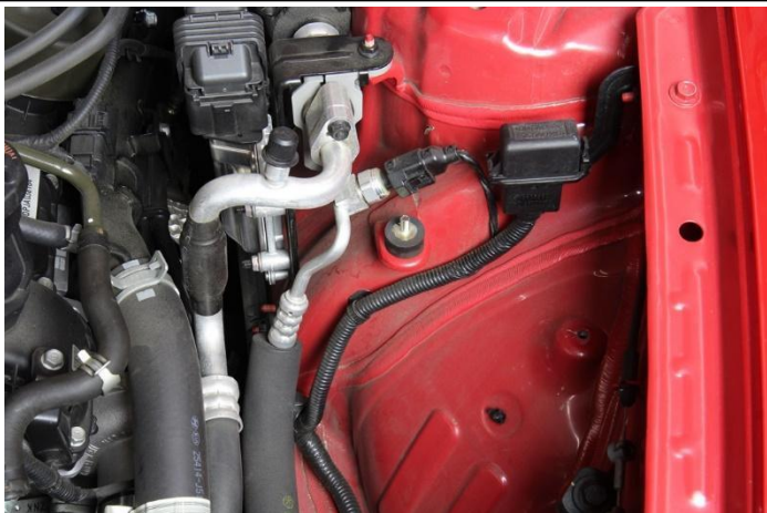
20. Install the 1/2" vibration mount onto the factory air box mount.
