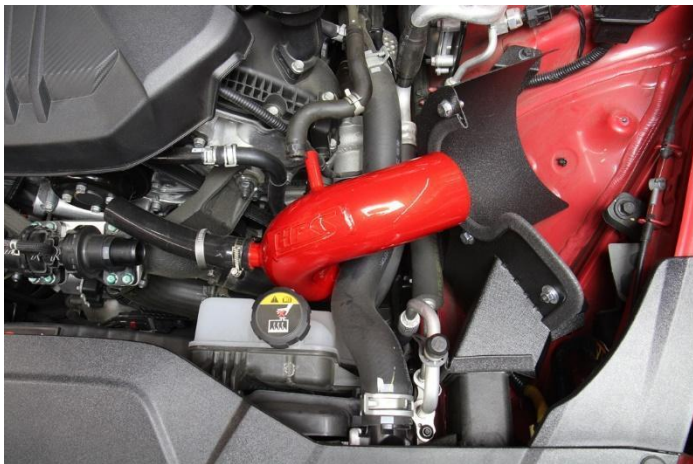
24. Insert the HPS intake pipe into the coupler. Adjust the intake pipe so that there is proper clearance around the intake pipe, then tighten the clamp securing the intake pipe to the coupler.
