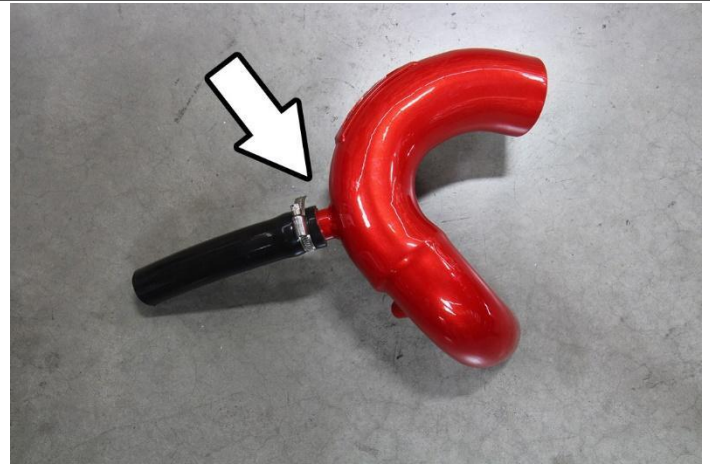
23. Prep the driver side HPS intake pipe by installing the shorter hose provided in the hardware kit onto the barb as indicated and secure the hose with the provided hose clamp.
