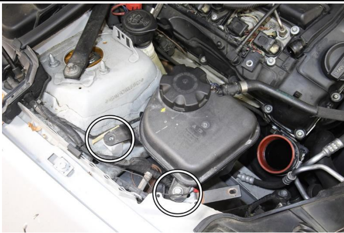
18. Remove the two 10mm bolts securing to coolant reservoir tank. Lift the tank and remove it from the grommet to have more space when installing the intake pipe.
