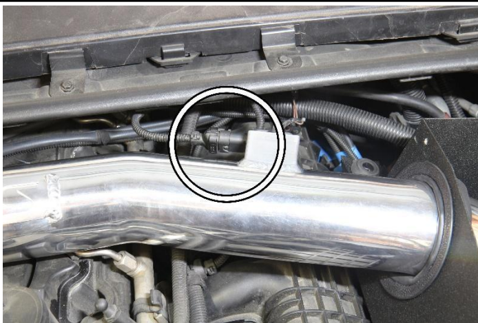
24. Re-connect the mass air flow sensor connector.
