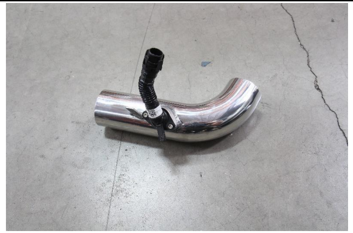
17. Install and secure the CCV hose onto the HPS intake pipe using the provided M5x12mm bolts.
