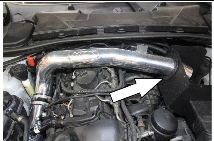
23. Insert the HPS intake pipe into the heatshield first, then secure the intake pipe into the coupler.
