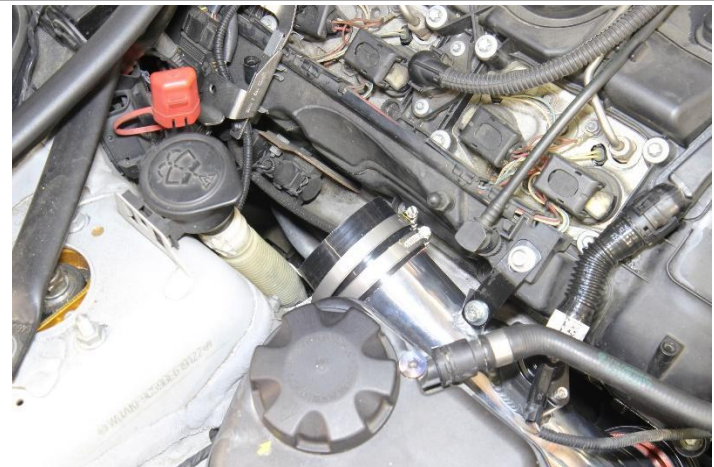
21. Install the 2" coupler along with the provided EMSC clamps onto the intake pipe. Be sure to leave enough space to secure the other section of the intake pipe.
