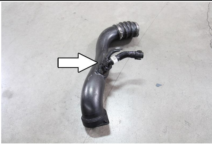
16. Remove the factory CCV hose from the intake tube.
