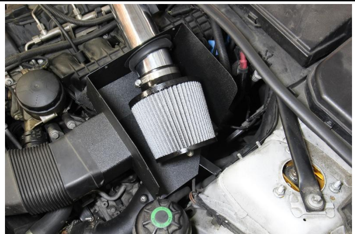
25. Install the provided HPS performance air filter.
