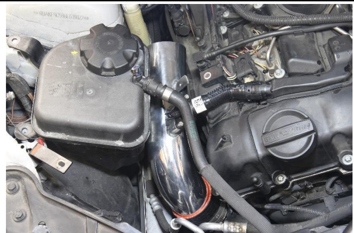
19. Insert the HPS intake pipe into the coupler and re-insert the CCV hose into the valve cover. Re-secure and mount the coolant reservoir tank.
