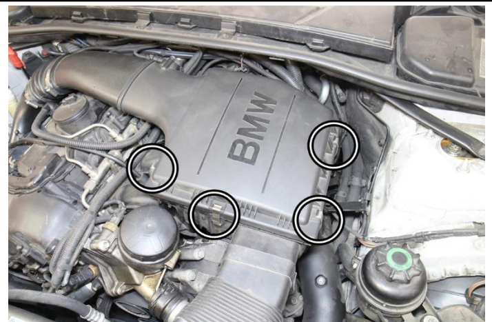
3. Disconnect the retaining clips securing the upper air box assembly.
