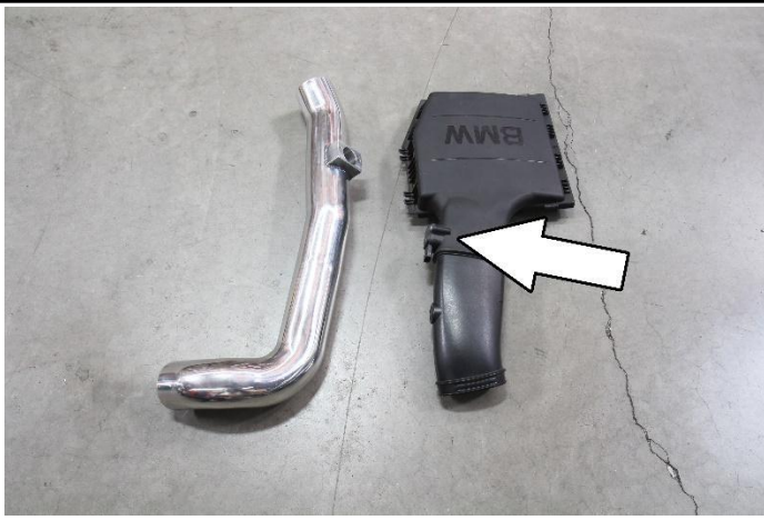
22. Install and secure the mass air flow sensor into the HPS intake pipe using the provided M5x12mm bolts.
