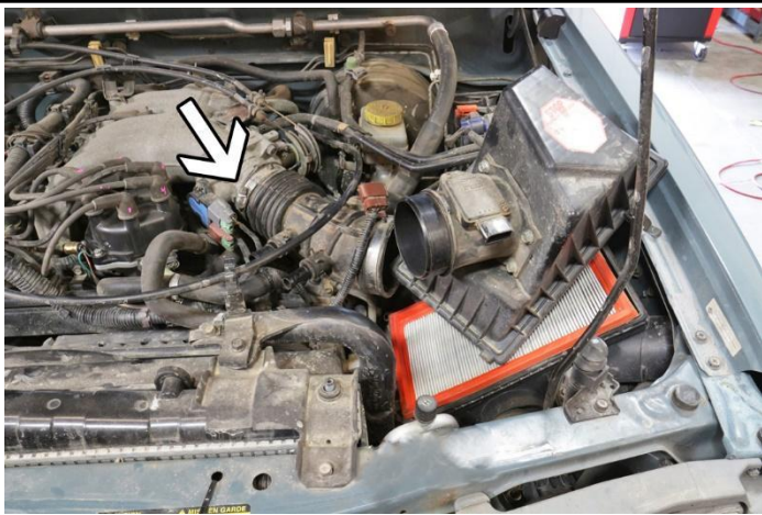
6. Remove the upper air box assembly from the vehicle. Loosen the hose clamp securing the intake tube from the throttle body.
