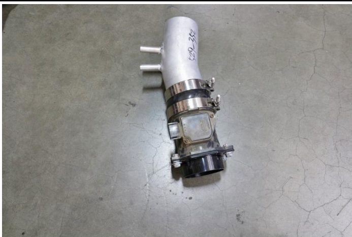
20. Install the reducer coupler along with the T-bolt clamps onto the MAF sensor housing and insert the HPS intake pipe into the coupler. Do not tighten the clamp for the intake pipe yet because the intake pipe will need to be re-positioned.
