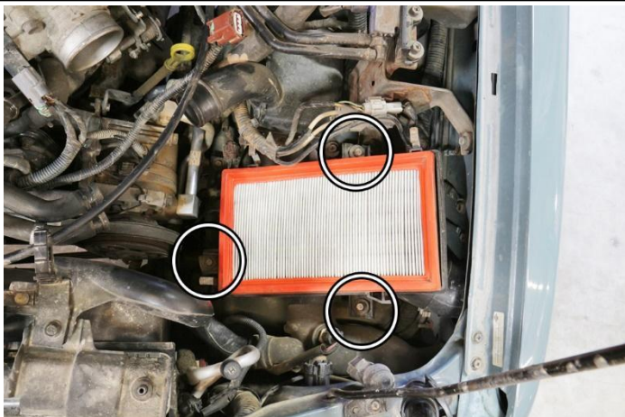
8. Remove the three bolts securing the lower air box assembly.
