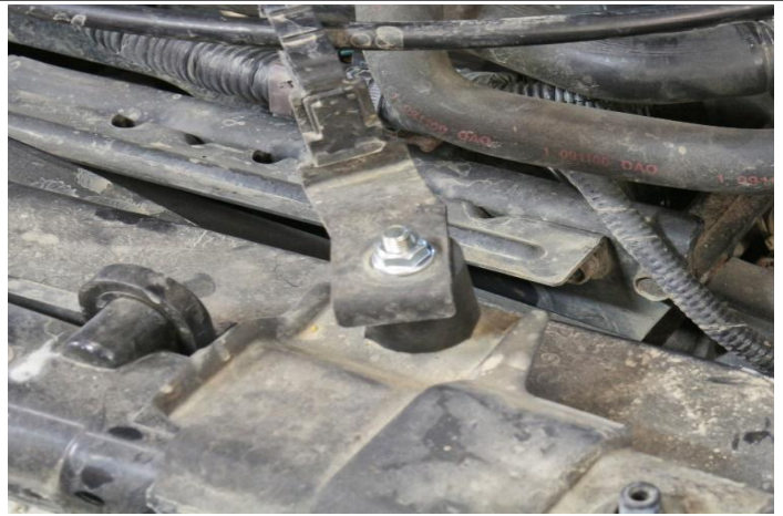
17. Install the cruise control bracket and secure the bracket with a nut and washer supplied in the hardware kit.
