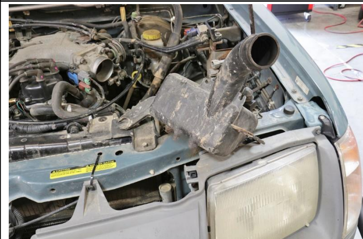
14. Remove the intake resonator from the vehicle.
