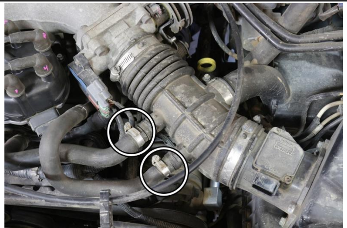
3. Using a pair of pliers, squeeze the hose clamps to loosen the breather hoses from the intake tube.
