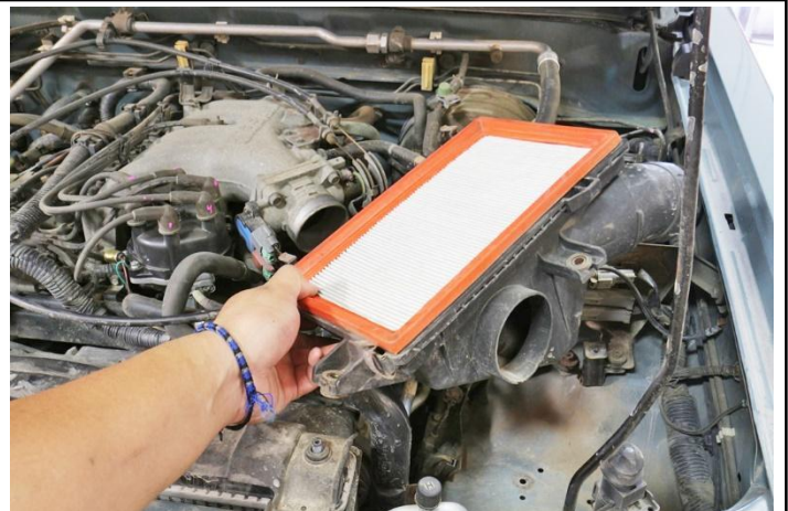
9. Disconnect the front resonator from the lower air box and remove the air box from the vehicle.
