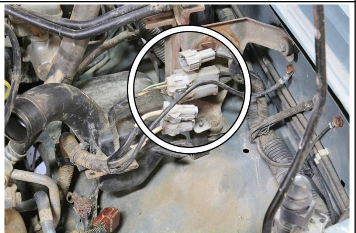
13. Disconnect the three electrical connectors in the image shown above.
