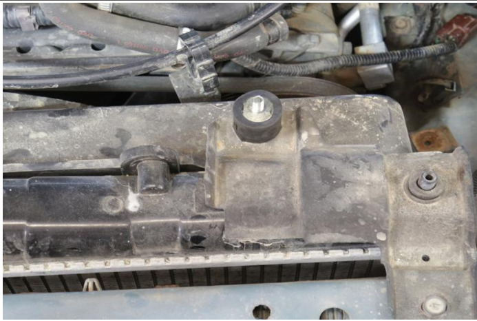
16. Install the 1" rubber vibration mount for the cruise control bracket.
