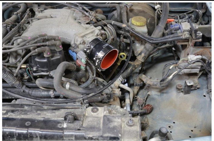
21. Install the reducer coupler onto the throttle body along with the T-bolt clamps included in the hardware kit.
