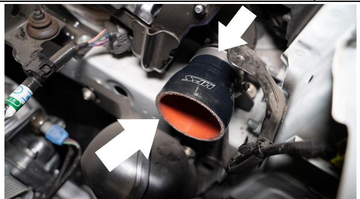
15. Install the reducer coupler HTSR-187-250-BLK using the provided EMSC-40-60 clamp onto the oem lower intercooler pipe.
