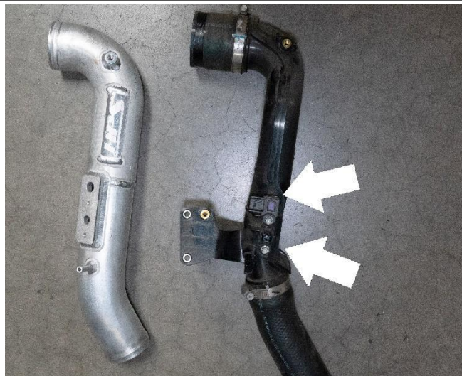
12. Uninstall the two sensors from the OEM intercooler pipe and transfer them onto the HPS intercooler pipe.
