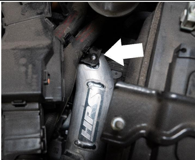
20. Install the provided M6 x 12mm bolt and washer to secure the heater hose bracket to the HPS upper charge pipe.
