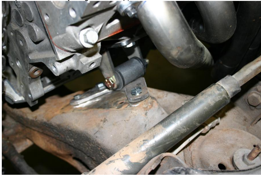
, (Detailed view of driver's side motor mount and frame bracket in chassis)
