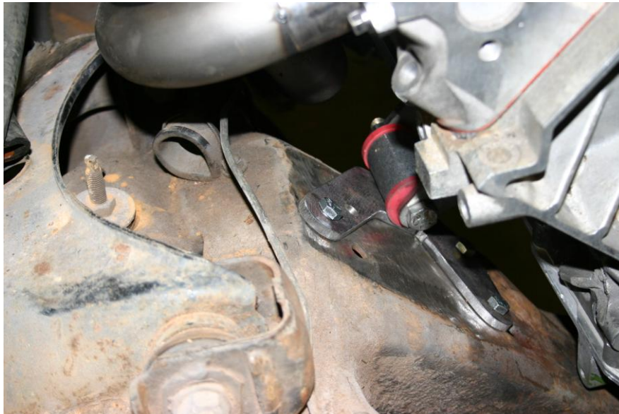
(Detailed view of passenger's side motor mount and frame bracket in chassis)
