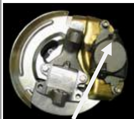
Bleeder Valves Up
