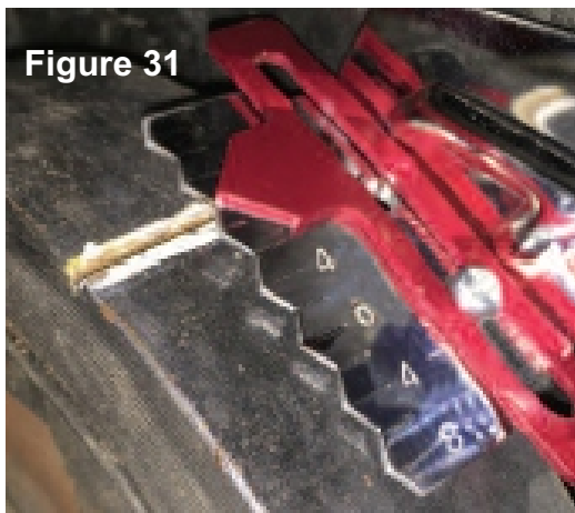
Timing Pointer at 10° before Top Dead Center
