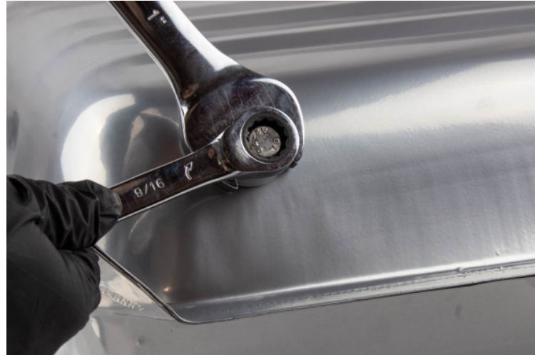
Twist bolt to collapse and set bung.
