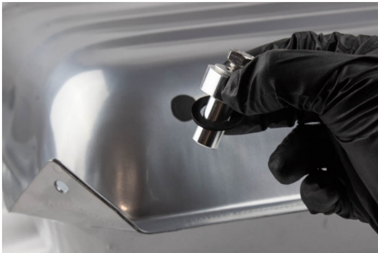
Insert fitting with gasket, screw and washer.
