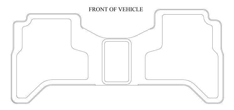
TO EASE INSTALLATION, ADJUST BOTH FRONT SEATS TO THEIR MOST FORWARD POSITION. WHEN LINER IS INSTALLED, REPOSITION SEATS AS REQUIRED.
