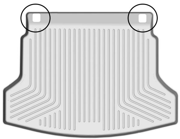
YOUR CR-V CARGO LINER IS DESIGNED TO ALLOW ACCESS TO THE FACTORY CARGO TIE DOWN HOOKS WITH THE LINER INSTALLED. TO ACCESS THE TWO HOOK LOCATIONS, SIMPLY USE A UTILITY KNIFE OR SIMILAR PRODUCT AND REMOVE THE MATERIAL FROM THE RECESSED AREAS ON YOUR LINER THAT CORRESPOND WITH THE HOOKS LOCATIONS (AREAS SHOWN ABOVE CIRCLED). USED THE EDGES FORMED BY THE RECESSED AREAS AS A TRIMMING GUIDE.
