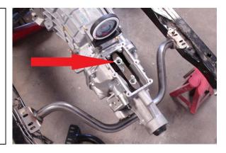
When you are sure your shifter is correctly positioned, apply a new bead of RTV sealer to the lip of the shifter cavity and mount the shifter by re-using the six, 5/16" bolts. Torque the bolts to 20 ft/lbs.
