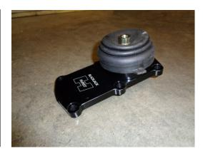
The shifter "body" will be in the forward position on the rear TKO shifter cavity. Make sure the pivot ball is positioned into the forward socket and that the white plastic bushing is still in place.
