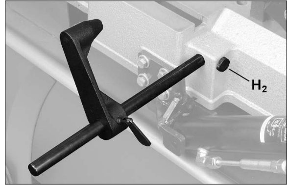
Figure 6-7: installing work stop (712 only)
