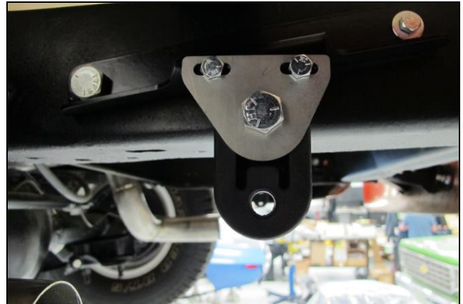
Driver's Side Dual Rear Exit System Tailpipe Hanger Installation Figure 3
