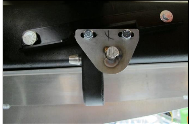
Driver's Side Dual Side Exit System Tailpipe Hanger Installation Figure 4
