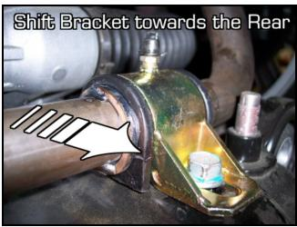
Use bracket with the 90° grease fitting for the front. Fitting points out board. Straight fitting is shown in pictures for prototyping.
