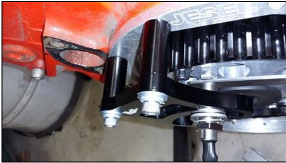
Figure 10: Adjusting Sensor Gap
