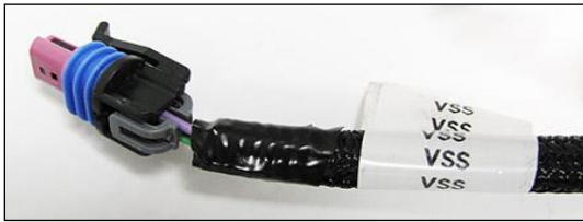
Figure 34 - Vehicle Speed Sensor
