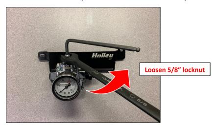
b. Turning adjustment screw clockwise increases pressure while counter-clockwise decreases pressure.
