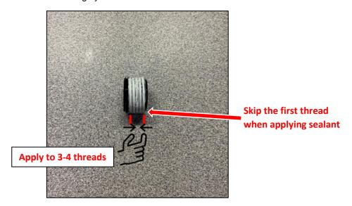
b. Apply Thread Sealant around entire diameter of 2-3 threads onto two NPT to AN Adapters (see Step 7a.)
