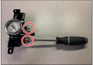
c. Mount Fuel Pressure Regulator on firewall using existing bolts with 10mm socket.
