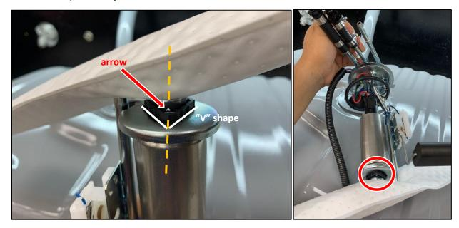
d. If aligned properly, the HydraMat's short end points in the 10 o'clock position and the long end in the 4 o'clock orientation. This maximizes the effectiveness of the mat and allows the short end of the mat to be tucked underneath the internal wall inside the tank.
