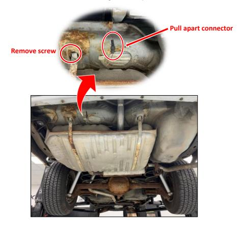
c.) Remove fuel line clamp bolt with **1/2**" **socket** and disconnect all (x3) hoses by relieving clamps with **pliers**. **NOTE**: Place fuel container underneath to prevent leakage onto floors.
