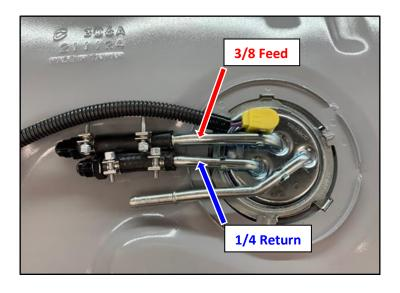
**NOTE:** For non-baffled fuel tanks, we recommend **Part #: 16-150**, 19mm Outlet Offset HydraMat, to greatly reduce the potential of air entering the fuel system and limit fuel starvation during hard cornering, braking acceleration, inclines, and low fuel conditions.
