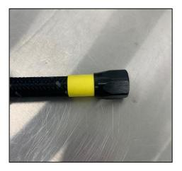
c. Lubricate inside of the hose and the fitting's threads with Earl's Assembly Lube.
