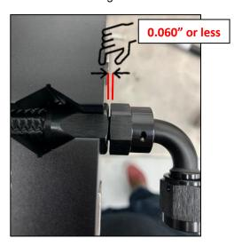
Check the tape to see if the hose end has pulled away from the hose, if it did back out more than  $\sim 1/16$ " out of the socket, try again by returning back to Step 12c.
