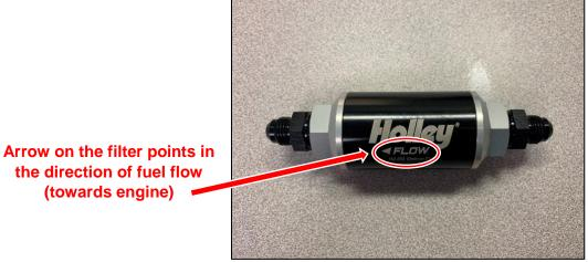
the direction of fuel flow (towards engine)
