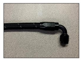
**NOTE:** Pressure test hose assembly to ensure no leaks. Further check the assembly by running the system at full pressure while you observe the hose, hose ends, and adapters for leaks.
