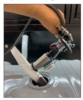
f. Lubricate the lock ring's O-ring with Earl's Assembly Lube.
