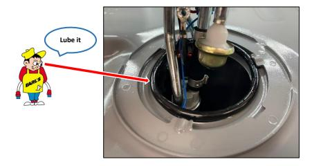
g. Seat lock ring and secure by rotating it clockwise with a Flat Head screwdriver and Rubber mallet.
