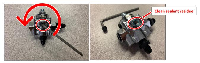
b. Apply Thread Sealant with PTFE around entire diameter of the leading threads on Fuel Pressure Gauge. Force the sealant into the threads to thoroughly fill voids.
