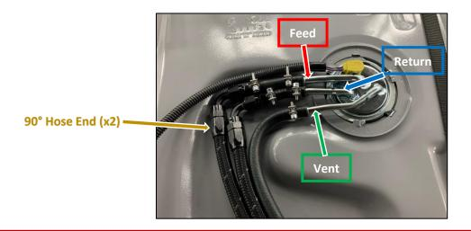
NOTE: The 5/16" vent hose can be replaced with 3 feet of 750055ERL and clamps: 750005ERL (not supplied).
