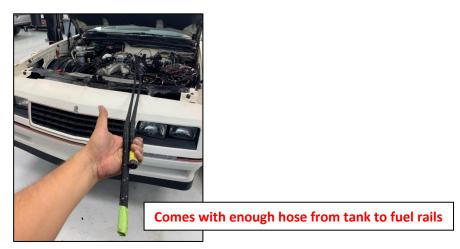
**NOTE:** Again, some extra fittings are provided but depending on what type of engine is being used and how fuel is being delivered, additional fittings may be necessary to adapt to the fuel injection system. Thus, we stopped at the engine bay to give as much flexibility to plumb the last connections onto the fuel rails or sniper.
