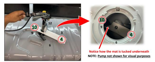
e. Slide long end of the HydraMat first along with tucking in the fuel sender float arm into the hole entrance. **NOTE: Be cautious to not tear the HydraMat while inserting into tank.**
