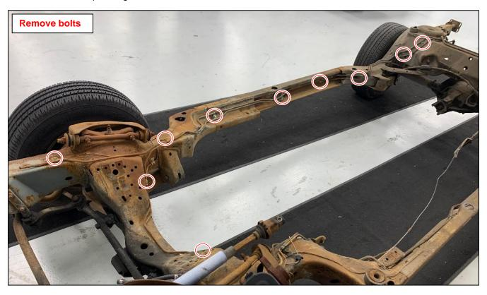
b. Completely remove all bolts and factory feed and return lines.
