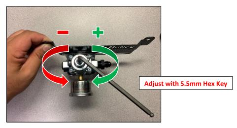
c. With fuel pump switched on, once desired pressure is achieved, tighten locknut with 5/8" wrench.
