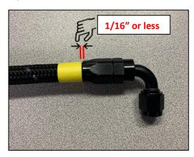
Remove the tape, and make sure your hose assembly is free of debris and thoroughly clean.
