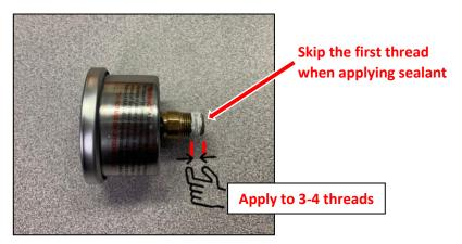
c. Install Gauge by hand first, then use a **7/16" open-end wrench** - turn clockwise to tighten.
