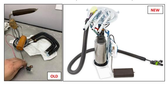
b.) OE Style Fuel Pump Module has Hose Barb inlets, so we will convert the 3/8" Feed and 1/4" Return to AN. Using the clamps, hose and the hose barb to AN adapter, tighten clamps with a **7mm socket**
