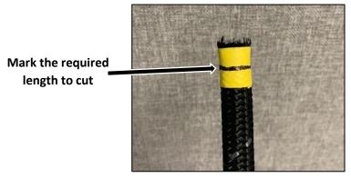
Not Acceptable: cut is not level, excessive fraying. Try again
