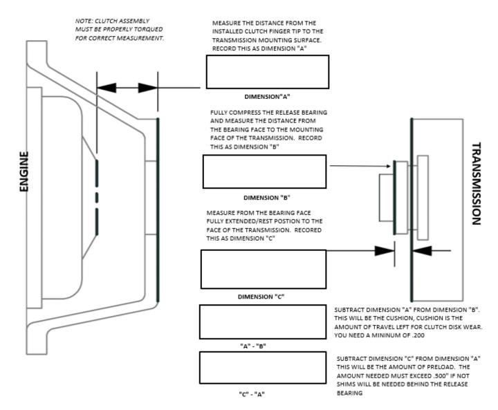
NOTE: All fasteners for the engine side or transmission side should be torqued between 35 and 45 ft./lbs. to maintain parallelism. It is more important that they are all torqued the same more than whether it is 35 or 45 ft /lbs.
