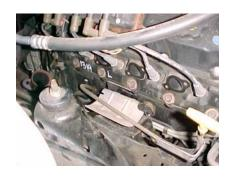
6. INSTALL SUPPLIED PASSENGER SIDE HEADER, GASKET AND SUPPLIED HARDWARE. TORQUE THE HEADER BOLTS TO 30-35 FTS. INSTALL THE 1/4" BOLT, LOCK WASHER AND NUT ONTO THE BRACKET FOR THE DIP STICK. MOUNT THE DIP STICK TUBE TO HEADER USING THE BRACKET. INSTALL SUPPLIED HEAT WRAP ONTO SPARK PLUG WIRE #10 FOR HEAT PROTECTION.
