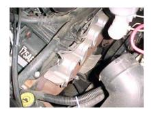
4. ONCE THE DRIVERS SIDE MANIFOLD IS REMOVED USE A WIRE BRUSH TO CLEAN HEAD SURFACE. INSTALL SUPPLIED DRIVER SIDE HEADER, GASKET AND HARDWARE. TORQUE HEADER TO 30 TO 35 FTS. AFTER DRIVERSIDE HEADER IS INSTALLED PUT SUPPLIED HEAT WRAP ON SPARK PLUG WIRES #7 AND 9 FOR HEAT PROTECTION. RE-INSTALL AIR CLEANER ASSEMBLY.
