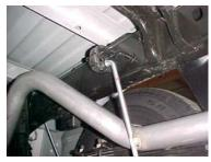
INSTALL PASSENGER SIDE TAILPIPE #C INTO MUFFLER 1-1/2" TO 2". USE CLAMP #G TO SECURE TAILPIPE TO MUFFLER. INSERT WELDED HANGER INTO RUBBER GROMMET. DO NOT TIGHTEN.
