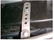
MEASURE 19 ½" FROM THE REAR OF THE FRAME AND USE THIS HOLE AND BOLT ON HANGER #G. USE THE 2<sup>ND</sup> HOLE FROM THE TOP.
