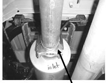
INSTALL HANGER # GIN FRONT OF THE MUFFLER AND INSERT INTO THE STOCK RUBBER GROMMETS. THEN INSTALL MUFFLER #B WITH INLET TOWARDS THE FRONT OF THE VEHICLE. USE A JACK STAND TO SUPPORT MUFFLER. DO NOT TIGHTEN.
