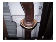
2. To remove your stock exhaust, unbolt the 2-bolt flange located in front of the muffler. Disengage the welded hangers from the rubber grommets. Use WD-40 to aid in this process. Do not remove or damage the rubber grommets as you will reuse them to mount your new system. Now, cut off tailpipe and remove exhaust. Do not throw away stock hardware.
