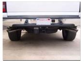
8. Install stainless steel tips #H. Clamp down. When you have everything in place, firmly tighten all bolts and clamps down securely. Use zip ties to secure fuel/brakes lines away from exhaust. Use stainless steel cleaner and a Scotch Brite pad weekly to prevent tip from discoloration.
