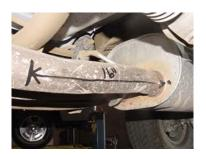
MEASURE 18" FROM THE REAR OF THE FRAME TOWARDS THE FRONT OF THE VEHICLE. USE THIS SLOT FOR THE 10" HANGER #K, INSTALL USING THE 1ST HOLE USE HARDWARE KIT PROVIDED.
