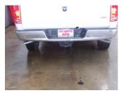
**9.** Install stainless steel tips #F. Clamp down. When you have everything in place, firmly tighten all bolts and clamps down securely. Use stainless steel cleaner and a Scotch Brite pad weekly to prevent tip from discoloration.
