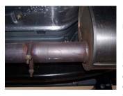
1. To remove the stock exhaust remove it from in front of the stock muffler. DO NOT REMOVE STOCK HEADPIPE. Disengage the welded hangers using WD-40 from the OEM rubber grommets. Do not damage or remove the rubber grommets as you will re-use them to mount your new system.
