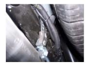
**6.** Measure 19½" from the rear of the frame. Use the third hole from the top to attach 10" hanger #H with bolt kit #I. DO NOT TIGHTEN.
