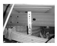
Remove the stock rear hanger from frame on passenger side. Install hangers # H to the frame using existing bottom hole where the stock hanger was mounted. Use the supplied nuts and bolts and mount the hanger through the fifth hole down from the top of the hanger. Repeat on the driver side.
