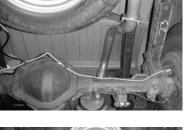
Slip the over axle tailpipes #C, #D into the outlets of the muffler no more then 1- 1/2" to 2" and attach clamp #G to passenger side and clamp hanger #I to driver side tailpipe. The driver side tailpipe will be routed over the differential between the frame and the shock. It will require some rotating of the pipe and possibly an extra person to help align the pipes when tightening the clamps. Attach hanger #H to tailpipes and attach with clamp #G.
