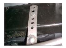
MEASURE 19 ½" FROM THE REAR OF THE FRAME AND ON THE DRIVERS SIDE USE THIS HOLE AND BOLT ON HANGER #F. USE THE 3<sup>RD</sup> HOLE FROM THE TOP.
