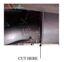
TO REMOVE STOCK EXHAUST, CUT OFF YOUR STOCK SYSTEM JUST IN FRONT OF THE MUFFLER AFTER THE WELD. LEAVE ALL RUBBER GROMMETS ON THE HANGER. USE WD-40 TO AID IN THE REMOVAL OF EXHAUST AND HANGERS.
