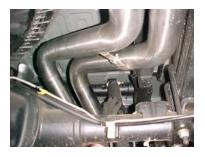
SLIDE PASSENGER SIDE TAILPIPE #C INTO MUFFLER 1-1/2" TO 2" AND INSERT WELDED HANGER INTO RUBBER GROMMET. USE CLAMP #F TO SECURE TAILPIPE TO MUFFLER. DO NOT TIGHTEN.
