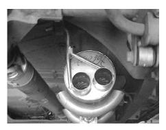
Install muffler #B with the inlet towards the converter onto the head pipes at least 1-1/2" to 2" using clamps #F. Use a jackstand to support. The outlets of the muffler should be at the 6 o'clock position.
