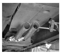
Bolt head pipe #A to the stock head pipe flange behind the converter reusing stock bolts and supplied gasket #I. Use a Hi-Temperature 02 sensor safe silicone on the gasket for a good seal. Insert welded hanger on driver side into rubber grommet. Re-install 02 sensor into head pipe. Apply a small amount of anti-seize on the threads. Do not tighten.
