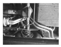
Install the passenger side over axle tailpipe #C onto muffler at least 1-1/2" to 2" using clamp #F to attach tailpipe. Insert welded hanger into rubber grommet. Do not tighten. Install Driver side over axle tailpipe #D into muffler at least 1-1/2" to 2" using clamp #F to attach tailpipe. Install hanger #G onto driverside tailpipe and insert into rubber grommet. Use Bolt Kit #H to secure both tailpipes together.
