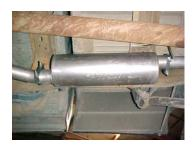
Install muffler onto head pipe 1-1/2" to 2" with the louvers facing towards the converter. Use a jack stand to support the muffler. Use clamp #G to secure the muffler to the head pipe. Do not tighten. Muffler inlet is looking into the louvers.
